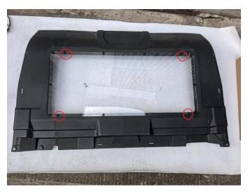
4. Lift the bed cargo and remove the plastic clips at both ends of the rear side of the frame for future use. Stick two sponge strips to the position of the rear pillar, as shown in the picture:
