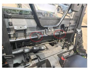
7. Fix the rear windshield to the rear pillar with four small straps, as shown in the illustration:
