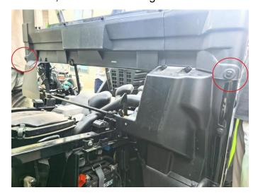
6. Remove the seat and fix the lower end of the rear windshield to the frame with two small straps.
