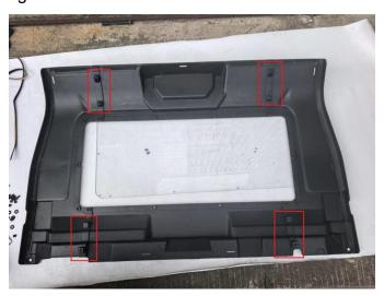
3. Install the transparent board onto the plastic part with ten M6\*16 hex socket screws, four M6\*20 hex socket screws and fourteen M6 lock
