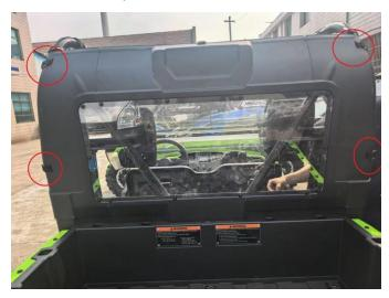
8. Fix the transparent board to the middle of the rear pillar with four M6\*16 hex socket screws, two M6 flat washers and four nuts through two iron brackets, and the installation is completed.
