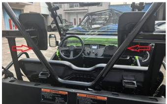
5. Fix the lower end of the rear windshield with two sets of plastic snap fasteners that just removed, as shown in the figure:
