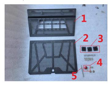
1. Combine Part 1 and Part 2 using 12 M5\*12 hexagon socket head cap screws and 12 M5 locknuts, as shown in the picture.
