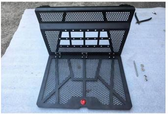
2. Install the hood button (Part 4) onto Part 2, as shown in the picture.
