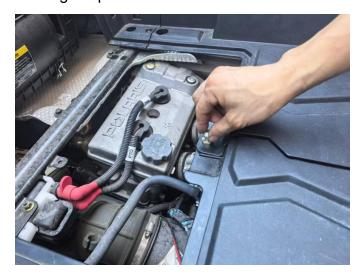
5. Secure the long screw (Part 5) to the lock hole of the cover using 2 M6 washers and M6 nuts, as shown in the picture.
