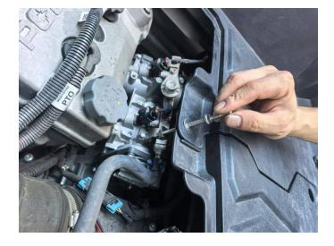
6. Snap Part 1 into the two notches, and the installation is complete.
