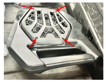
2. Open the original vehicle's driver door, remove the screws and snap fasteners securing the outer door trim panel, and then detach the outer door trim panel. As shown in the picture:
