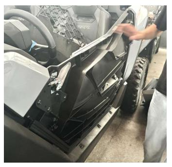
3. Prepare a 6MM drill bit, and drill holes sequentially at the pre-marked points on the original door panel. Then, install the assembled speaker pod on the inner side of the door panel, and secure it with the provided screws from the outer side of the door panel. Finally, reattach the outer door trim panel to its original position. (Install the speaker pod on the other side using the same method.) As shown in the picture:
