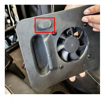
3. Connect the extended wiring harness to the switch according to the sequence shown in the image, and connect the other plug to the wiring harness plug on the fan. Finally, reinstall the inspection hole cover back onto the vehicle. As shown in the figure:
