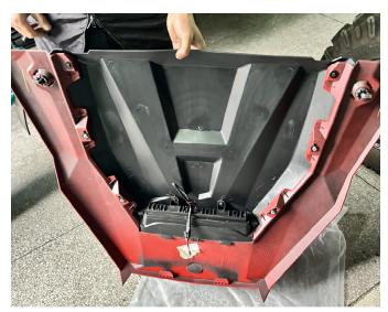
2. Prepare the extension cable that comes with the product, cut the white extension cable into two cables of equal length, connect them to the wiring harness of the hood-mounted spotlight (connect the red wire to one extension cable and the black wire to another extension cable, and ensure proper insulation at the connection points). Then, route the two
