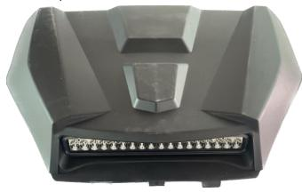
1. First remove the original hood scoop, replace and install the new inner hood, secure it with M5\*20 and M6\*19 self-tapping screws and washers, and then reattach the hood to the vehicle. As the picture shows:
