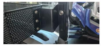
5. Secure the upper end of the mounting bracket to the front A-pillar with two self drilling screws, and the installation is complete.
