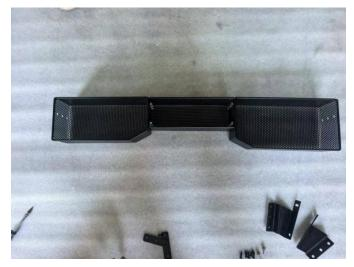
3. Use 4 pieces of M6\*16 hex socket screws, 4 pieces of M6 lock nuts, and 2 pieces of iron brackets (part 4) to install the left mounting bracket and the right mounting bracket to both ends of the storage box respectively, do not tighten the screws, as shown in the figure.
