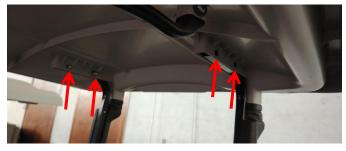
4. Use the original screws removed earlier to install the assembled storage box in the corresponding position and tighten the screws. Note: The side of the storage box with the notch should face the front of the vehicle.
