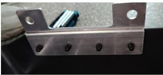
3. Remove the original screws from the rear of the roof and keep it for later use.
