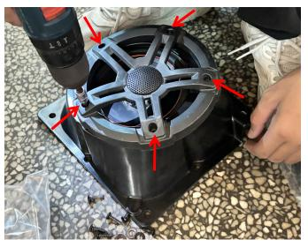
3. Install the speaker bracket under the vehicle dashboard and secure it using M5\*20 self-tapping screws and flat washers. (Install the other side in the same manner). As shown in the figure:
