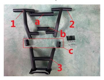
1. Assemble part 1, 2, and 3 using 8 M8 \* 50 hex screws and 8 M8 jam nuts, with one sleeve a, one sleeve b, and two sleeves c. As shown in the picture:
