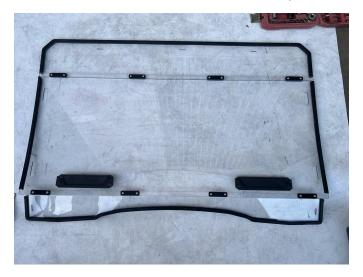
2. Use two small straps and four large straps to secure the front windshield to the front pillar, then use three small straps to secure the upper end of the front windshield to the front crossbeam, and complete the installation.
