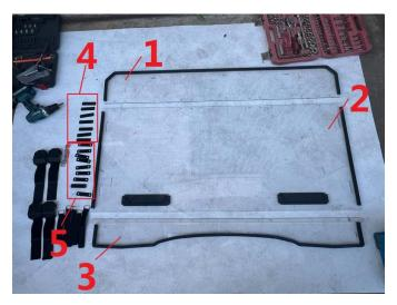
1. Assemble PC board 1, PC board 2 and PC board 3 with 16 M6\*20 hexagonal screws, 16 M6 locknuts through 8 pressure plates 4 and 8 pressure plates 5. Pressure plate 4 is mounted on the outer of PC board. As shown in picture:
