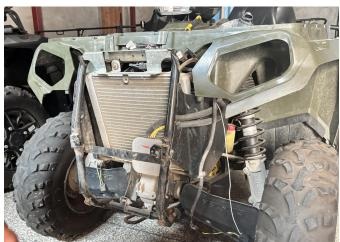
5. Remove the original headlights from the front fascia and transfer them to the new front fascia. The original metal clips must also be relocated to the new fascia in their original positions. Then, install the new front fascia back onto the vehicle. Finally, reattach the previously removed lower plate and storage box cover. As shown in the figure:
