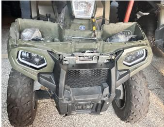
4. Remove the original front fascia and lower cover of the vehicle. As shown in the figure:
