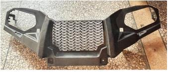
3. Open the front body rack cover of the vehicle and remove it. As shown in the figure:
