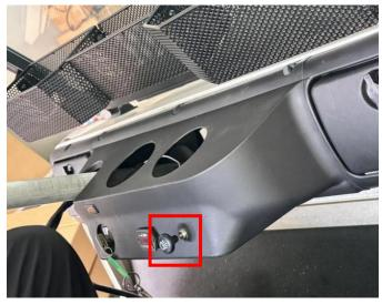
5. Use the original self-tapping screws to reinforce the power indicator light and properly place the matching cup holders. Then, use a 3.2MM drill bit to drill holes in the vehicle sequentially according to the screw hole positions at the edge of the dashboard. After completion, use a M4 tap to thread the screw holes. Finally, use the matching screws to fix the dashboard. As shown in the figure.
