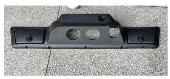
3. First, remove the original steering wheel, gear handle, and decorative panels from the dashboard of the vehicle. Then, install the assembled dashboard onto the vehicle (temporarily unfixed), and properly install the vehicle's original keyhole and power indicator onto the dashboard. As shown in the figure:
