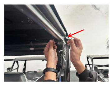
3. Install the bracket onto the roof using the provided clamps, securing it with M6\*16 and M10\*60 screws and nuts. As shown in the illustration:
