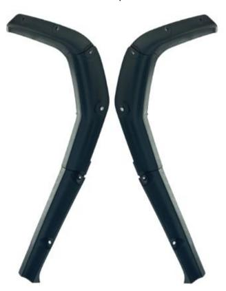
1. Use the self tapping screws provided with the product to assemble the separated fender flares into a whole. As shown in picture:
