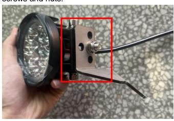
3. Unscrew the two fixing screws at the A-pillar. Re-pass provided screws to the A-pillar screw holes, then add an aluminum liner tube to each of the two screws, and finally install the pod light bracket, adjust the angle of the pod light, and use nuts to lock it. (NOTE: Route light wiring harness through adjacent gaps to reach headlight before fixing light.) As the picture shows:
