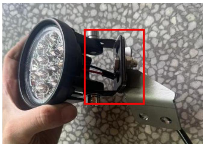
3. Unscrew the two fixing screws at the A-pillar. Re-pass provided screws to the A-pillar screw holes, and finally install the pod light bracket, adjust the angle of the pod light, and use nuts to lock it. (NOTE: Route light wiring harness through adjacent gaps to reach headlight before fixing light.) As the picture shows:
