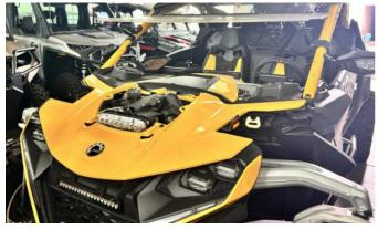
4. Remove the rear protective cover from the vehicle headlight and disconnect the wiring harness connectors for the headlights and daytime running lights.
