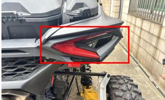
4. Remove the steel clips from the original trim panel and transfer them to the new trim panel. Then reinstall the new trim panel onto the vehicle and secure it using the original vehicle screws. (Replace and install the trim panel on the other side using the same procedure.)
