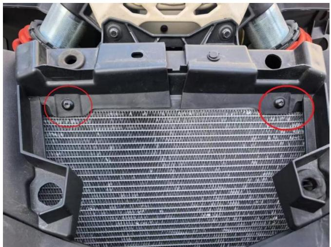
5. Unscrew the headlight bolts, disconnect the wiring harness connector, and remove the front fascia panel.
