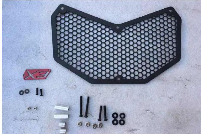
2. Attach the letter X3 to the mesh plate using two M4\*12 hex socket screws and two M4 lock nuts.
