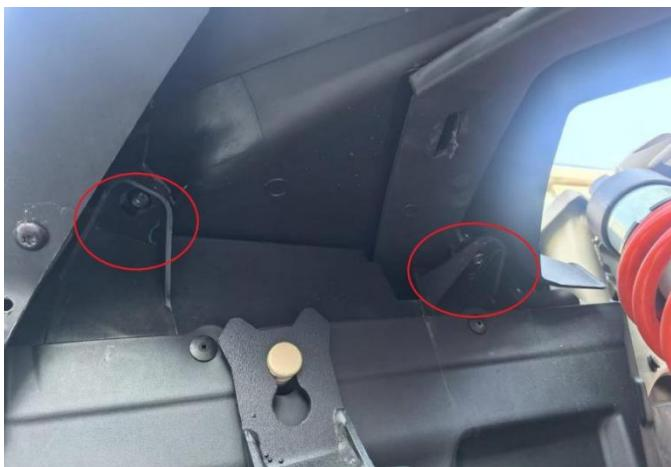
4. Remove the two screws at the front of the vehicle (keep the screws for later use), open the front cover plate, and remove the two screws connecting it to the radiator frame (keep the screws for later use).
