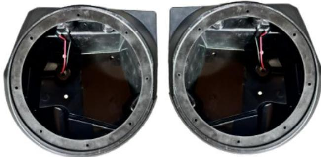
3. First, distinguish the left and right sides of the speaker brackets. Next, position the speaker brackets at the corresponding locations on the vehicle. Then, prepare a 6mm drill bit and drill holes sequentially according to the screw hole positions on the speaker brackets.
