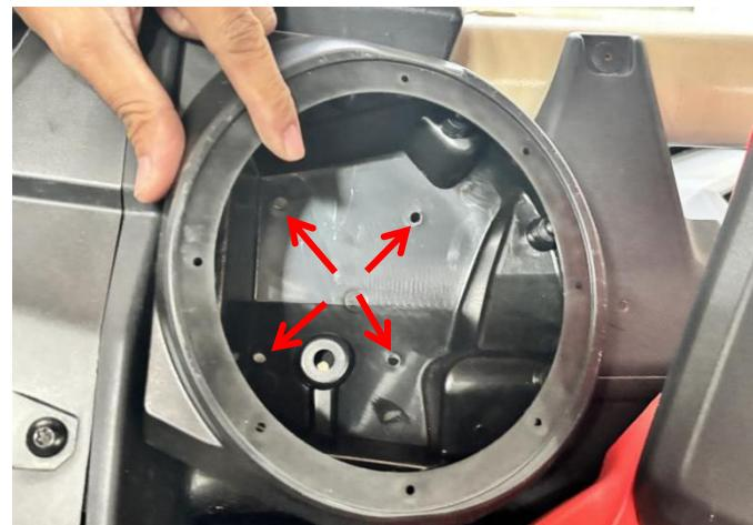
4. After drilling, secure the assembly using M6\*20 screws and matching flat washers. Finally, attach the speaker you provided to the bracket using the included self-tapping screws (the wiring harness of the speaker needs to be connected by yourself). Install the other speaker bracket using the same method described above.
