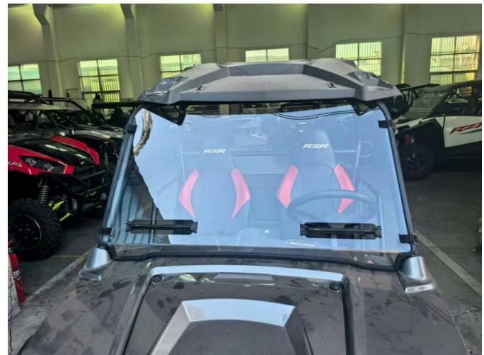
2. Secure the upper end of the full windshield to the pillars using 2 small straps.
