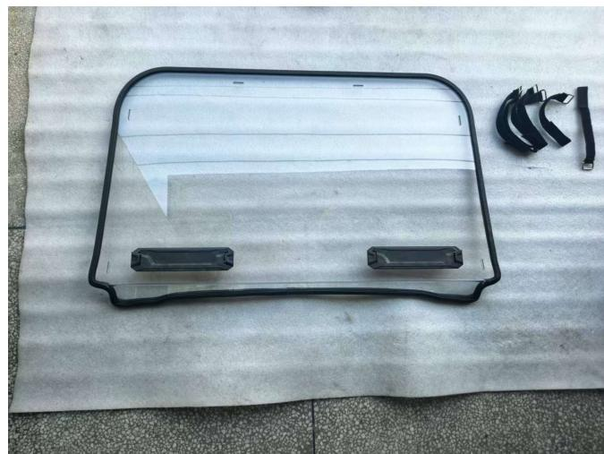
1. Secure the full windshield to the front pillars using 4 small straps.
