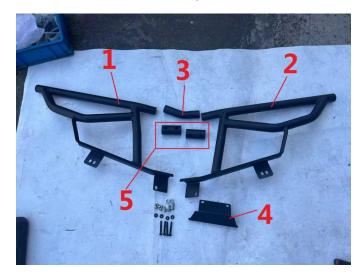
1. Assemble components 1, 2, and 3 using two sleeve components 5, secured with four M8 x 50 hexagon socket screws and M8 lock nuts. As shown in the picture:
