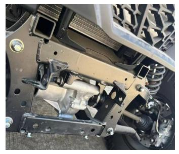
3. Using two M10 x 20 hexagon socket head cap screws and two M10 lock nuts, assemble the removed front lower bumper and upper bumper via mounting bracket 4. As shown in the picture:
