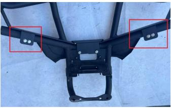
5. Using the four screws removed from the original vehicle's front lower bumper, fit the complete front bumper to the frame. Tighten the screws to complete the installation.
