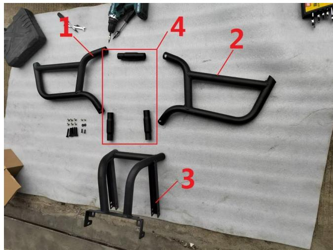
1. Use six M8\*45 hexagon socket head screws and six M8 lock nuts to assemble component 1, component 2 and component 3 through three sleeves 4. As shown in the picture:
