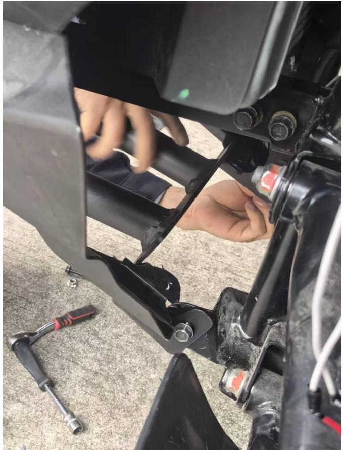
3. Fix the front bumper to the frame with the six screws that have just been removed, as shown in the picture. Use two M6\*20 hex screws, two M6 flange lock nuts and two M6 flat washers to fix the arrow position (the original plastic buckle position).
