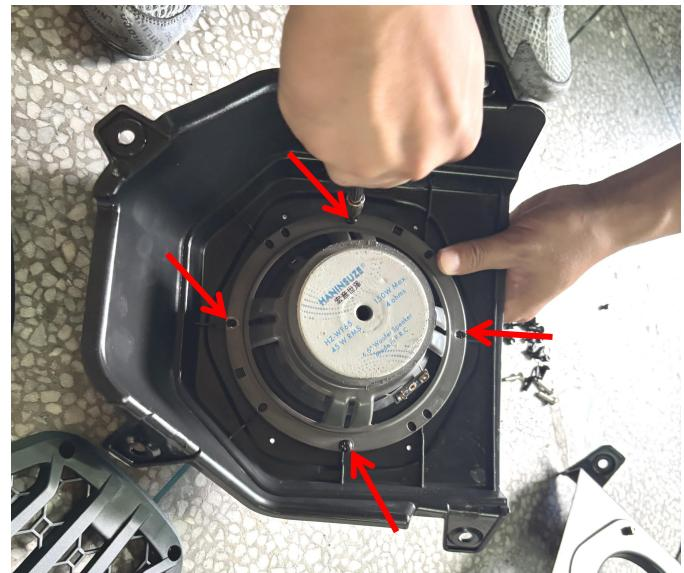
2. Prepare a white marker and a 5.2mm drill bit. First, position the speaker bracket beneath the original dashboard in the corresponding location. Then use the marker to mark the two mounting holes beneath the bracket. After removing the speaker bracket, use the drill bit to drill holes at the marked locations. As shown in picture:
