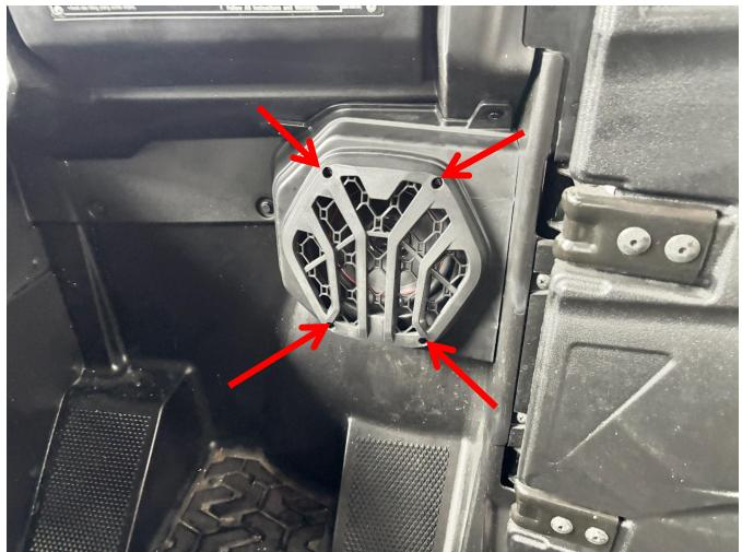
3. Reinstall the speaker bracket onto the original vehicle using the screws, nuts, and self-tapping screws provided with the product. Finally, secure the decorative outer frame of the speaker bracket. (Repeat the same steps for the other side.) As shown in picture:
