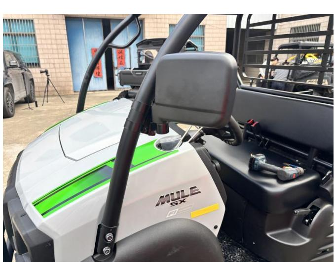
3. Finally, install the side mirror on the bracket using matching screws, lining tubes, flat washers, and nuts for fixation (the other side can be installed in the same way as above). As shown in picture:
