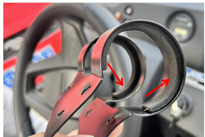
2. Insert the installation bracket with the sponge strip attached onto the original A-pillar of the vehicle (the height can be chosen independently), and then use the matching screws, lining tubes, flat washers, and nuts to fix it. As shown in picture:
